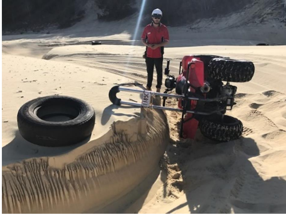
Figure 1. Observation of typical low speed roll over with OPD resting on sand bank
