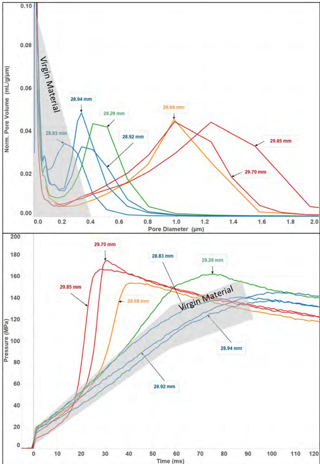
Figure 10. Pore size distribution (top) and corresponding closed chamber pressure-time histories (bottom) for selected 2004 10.8 g wafers. (Curves with the same color in each plot represent materials from the same inflator identified by OD of the MIP tested wafer. The gray area represents the typical range of behavior of virgin materials.)
