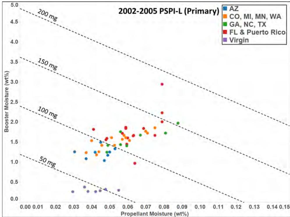
Figure 3. Moisture content in the primary chamber propellant and booster (3110 material only) in PSPI-L inflators from 2002-2005 vehicle model years. (The dotted lines indicate the total moisture in the 2004 propellant and 3110 booster materials.)
