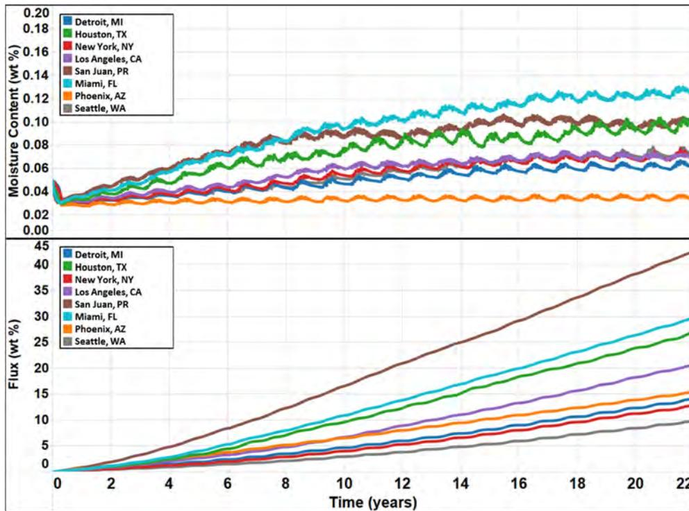
Figure 19. Moisture content and moisture flux in the 2004 propellant material over time in a PSPI-L primary chamber with outdoor exposure in different cities across the United States.
