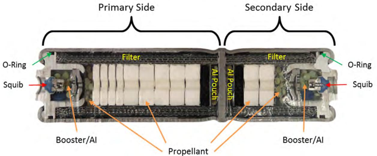
Figure 1. Cross-sectional view of a PSPI-L inflator. Other passenger inflator types characterized in this work have similar features.
