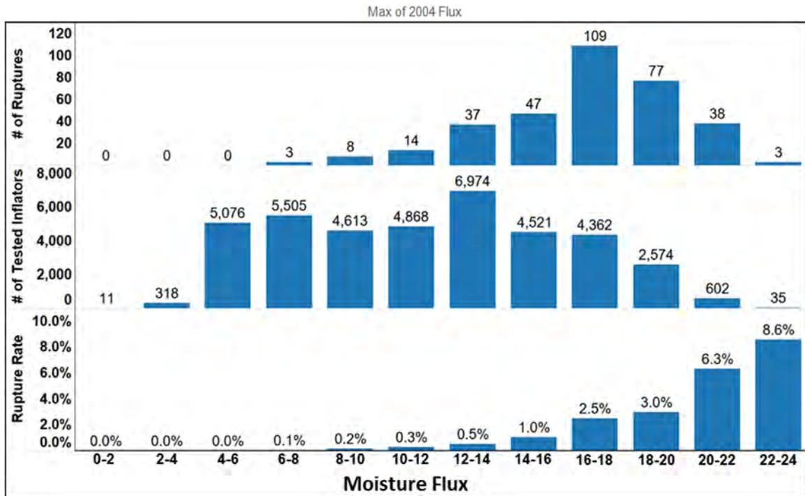
Figure 21. Rate of PSPI-L inflator rupture in Takata testing as compared to the calculated 2004 propellant moisture flux. No ruptures occurred below 7.6% moisture flux as calculated using the parameters specified in the model.
