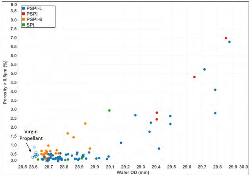
Figure 9. MIP porosity above 0.5  $\mu\text{m}$  pore diameter versus OD for propellant wafers from different inflator designs. (The nominal OD for virgin wafers is 28.6 mm, as denoted by the hollow circles.)
