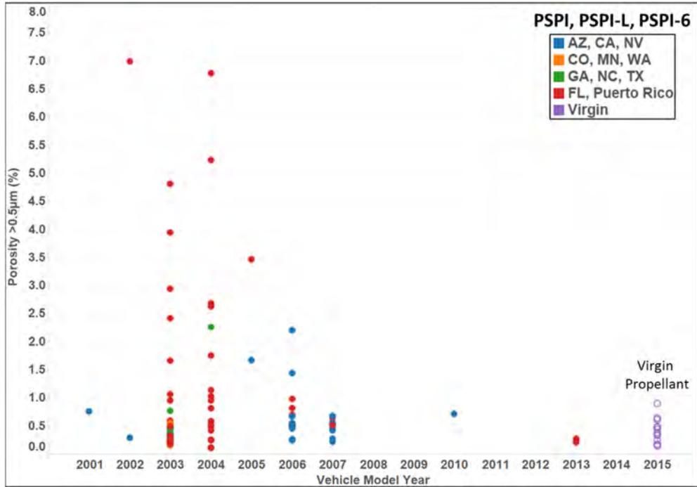
Figure 8. MIP porosity (for pore size above 0.5 µm) in 2004 wafers from inflators of different model year and location of operation.
