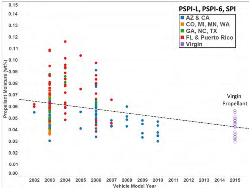
Figure 4. Moisture content in the 2004 propellant in various field returned inflators. (Data from the primary and secondary chambers are shown. The dotted line shows a linear fit through all of the presented data.)
