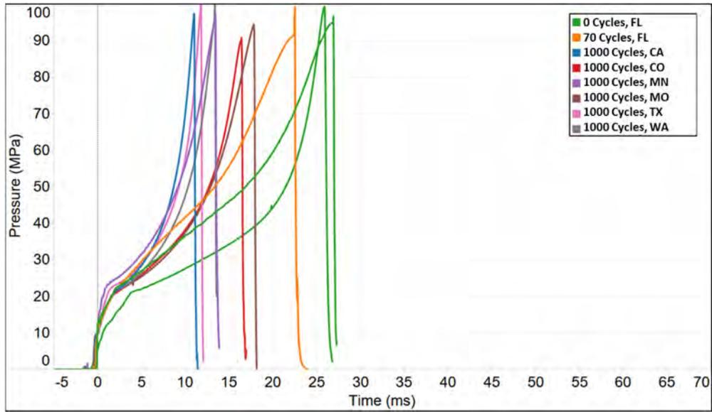
Figure 12. Measured pressure-time histories for ruptured field returned PSPI-L inflators. (All ruptures occurred in the primary chamber. Cycling conditions were 2-80°C, 4 hours/cycle.)
