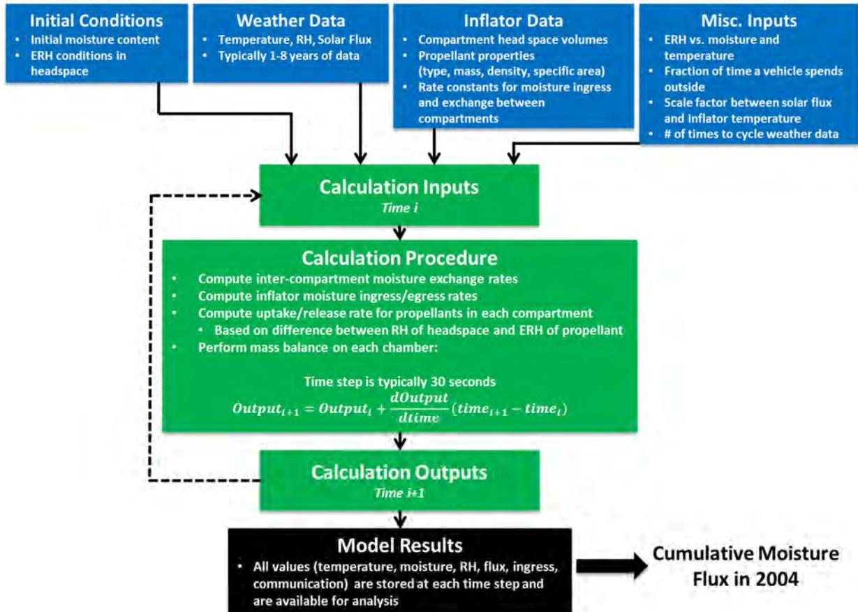
Figure 18. Summary of the inputs, assumptions, and calculation procedure in the Exponent numerical model for tracking moisture movement in the inflator.
