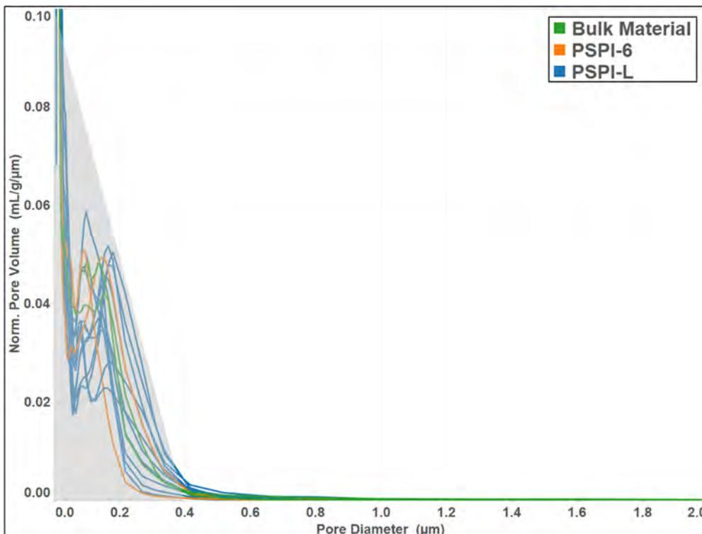
Figure 5. MIP pore size distribution for a variety of virgin 2004 propellants. (Bulk material refers to pressed 2004 propellant received directly from Takata prior to assembly into any inflators. Similarly, test material for PSPI-6 and PSPI-L was extracted from virgin inflators.)
