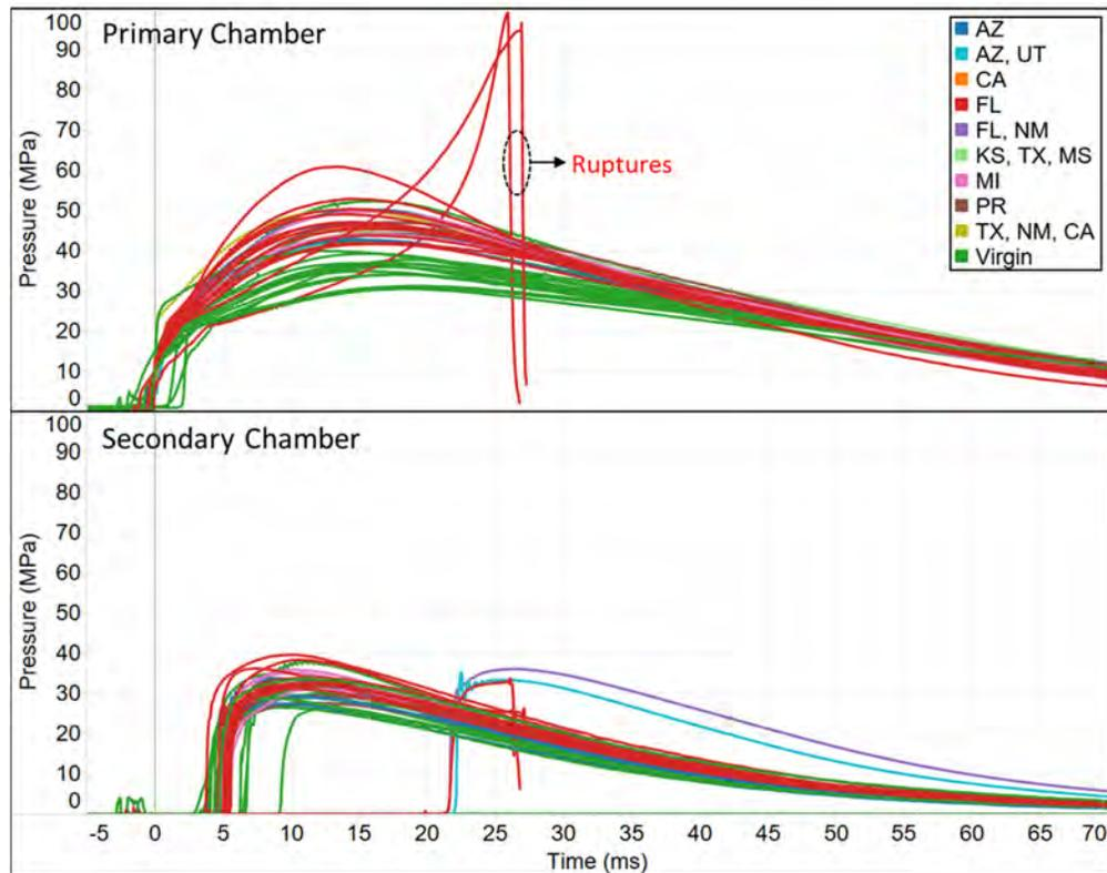
Figure 11. Measured pressure-time histories for virgin and field returned PSPI-L inflators. Data were acquired with various time delays between the deployment of the primary and secondary chambers.
