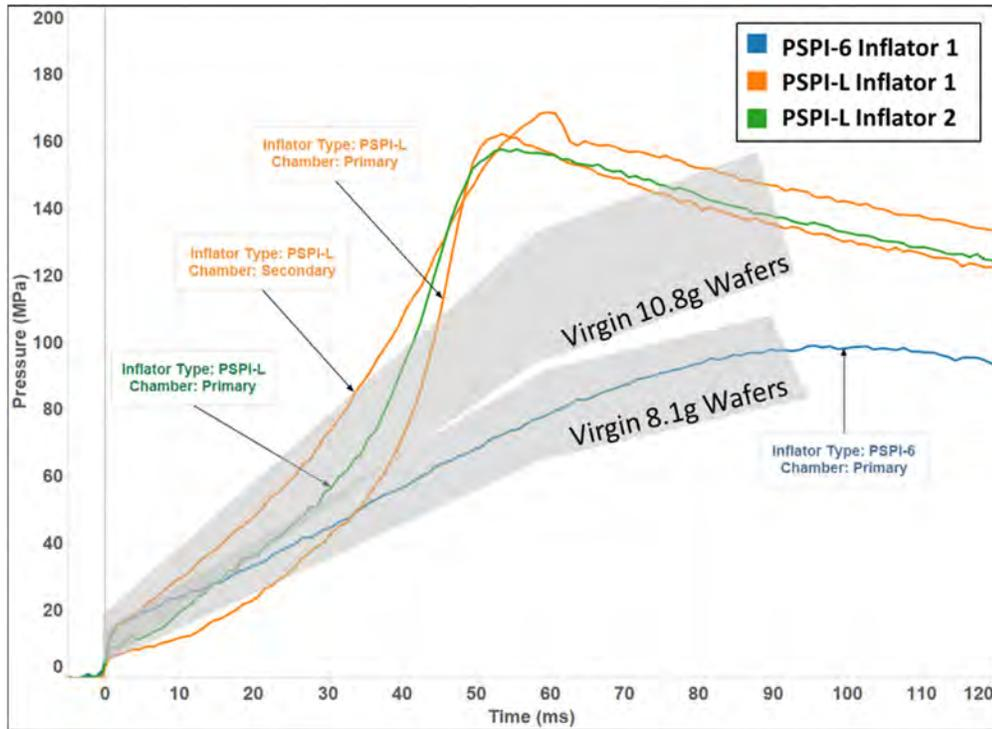
Figure 14. Closed 57 mL chamber pressure-time history of virgin inflators cycled 800 times (2-80°C, 4 hours/cycle). (10.8 g wafers are present in PSPI-L inflators and 8.1 g wafers are present in PSPI-6 inflators.)
