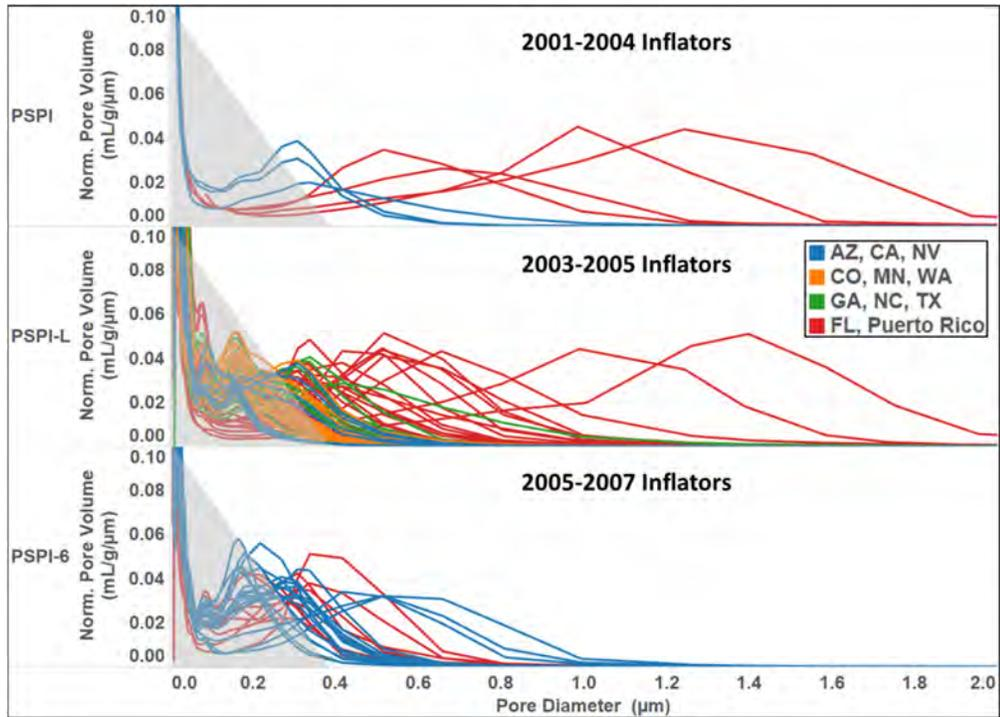
Figure 6. MIP pore size distribution for 2004 propellant wafers from field returned inflators. (Data from the primary and secondary chambers are shown. The gray region illustrates the range of typical pore size distribution in virgin materials.)
