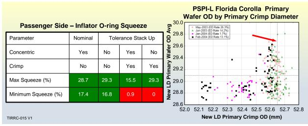
Figure 14. Passenger Inflator Primary Crimp Data.
