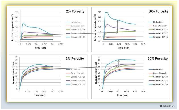
Figure 12. Impact of Porosity and Permeability.
