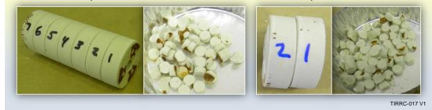
Figure 16. Examples of Fused Wafers and Tablets.
