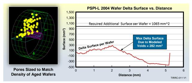
Figure 10. Closed Pore Impact on Burning Surface.
